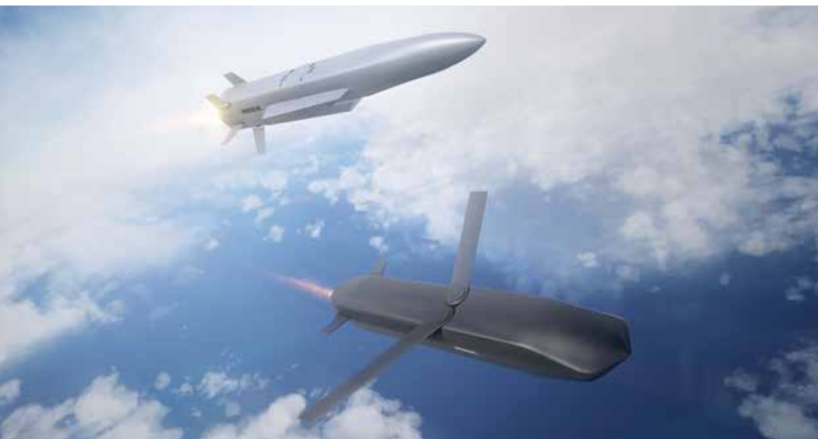
◀ Artist's impression of the two effectors being developed under FC/ASW. These comprise the ramjet-powered supersonic cruise missile known as RJ10 (top), and the low-observable turbojet-powered subsonic cruise missile TP15 (bottom). [MBDA]
