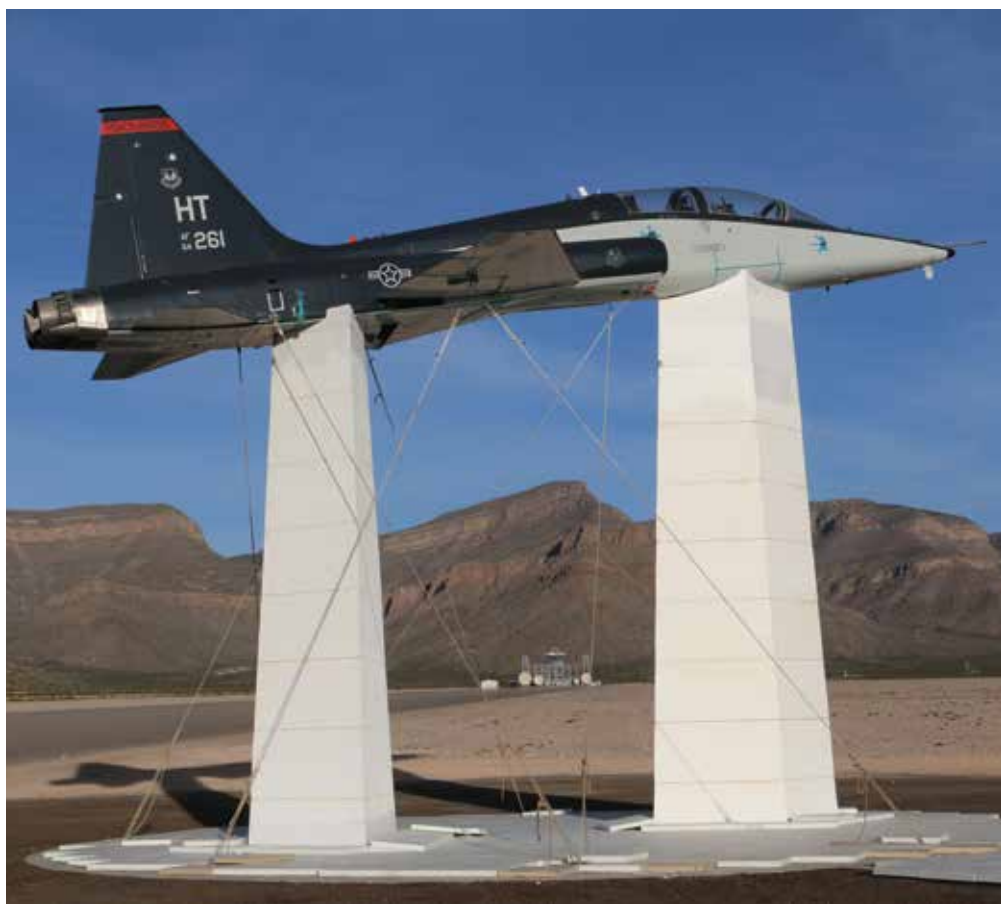
▲ Air forces and aeronautical engineers spend considerable time and effort to ascertain the visibility of aircraft to radar. Testing regimes can include mounting aircraft on plinths like these shown here and illuminating the aircraft with representative radar signals from a myriad of angles to ascertain RCS size. [USAF]
