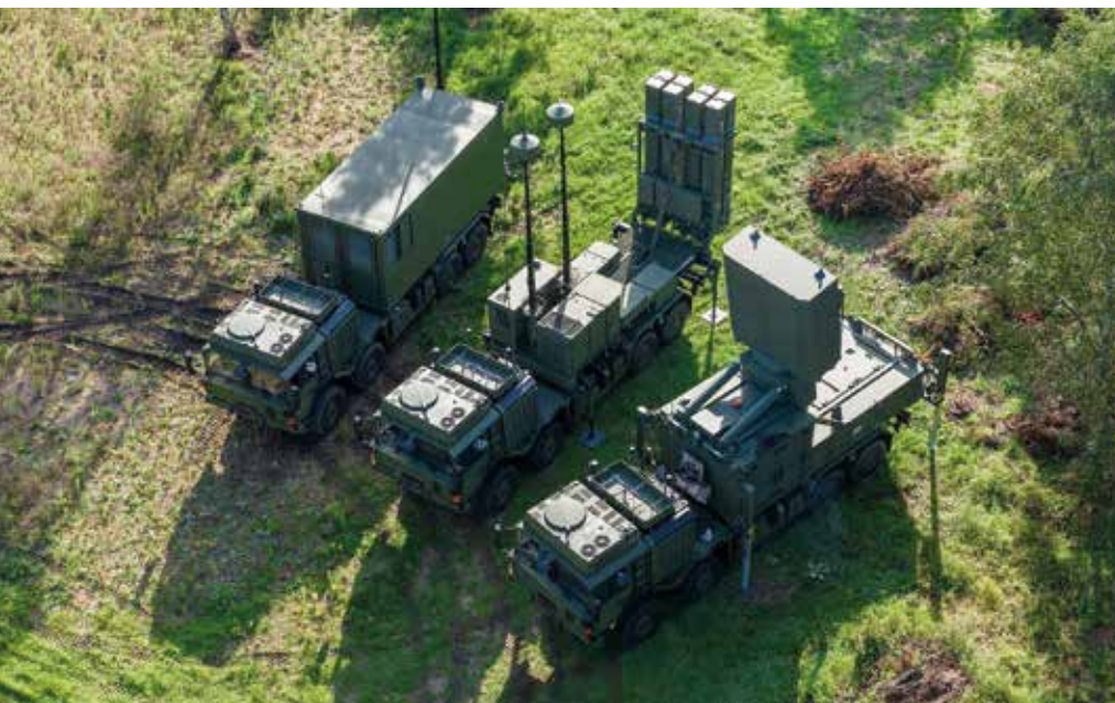
▲ IRIS-T SLM key system components viewed from above, consisting of the command post (left), transporter, erector, launcher (TEL; middle), and radar (right). This system forms the MRAD component of ESSI. [Diehl Defence]
