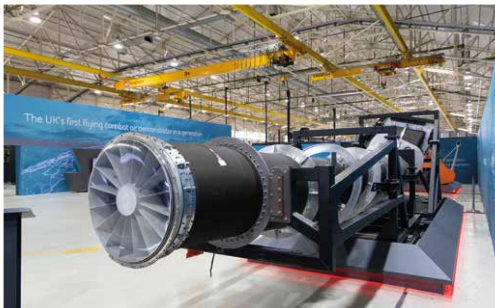
▲ One of the Combat Air Flying Demonstrator's engine ducts – looking forward from the point where it will attach to the front of an EJ200 engine. Its length and serpentine nature are apparent. [BAE Systems]
