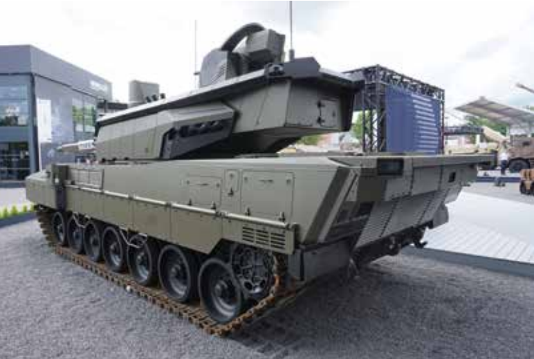
▲ A mock-up of Thales' Diamant hard-kill APS was shown on the EMBT-ADT 140 prototype shown at Eurosatory 2024. It is shown here as a black strip of effector modules running along the top of the turret, with radars at the turret corners. [Mark Cazalet]
