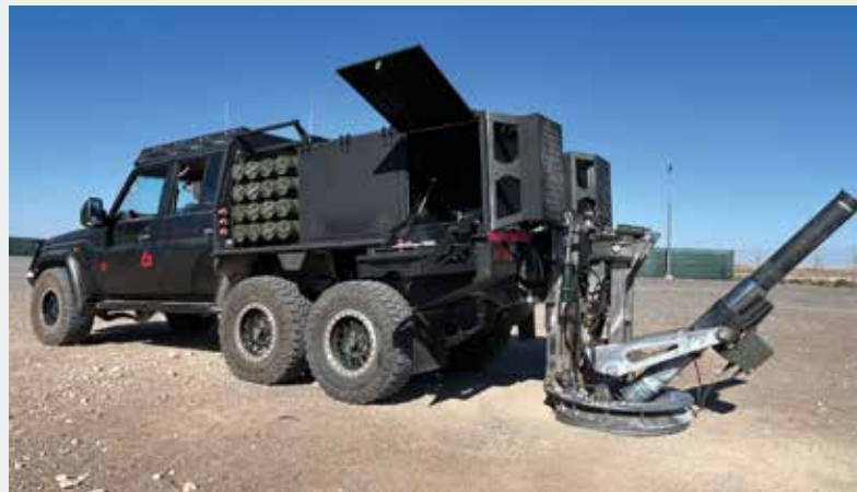
▲ The GDAMS 120 mm mortar system on Tac-6 6x6. [ST Engineering]
