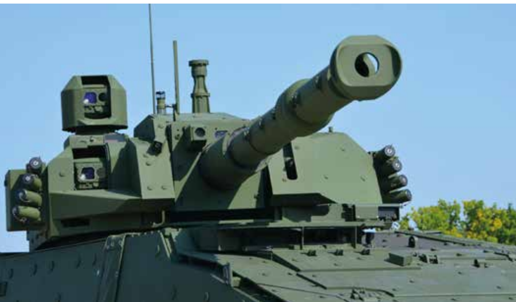
▲ A 3105 mobile gun system on the Boxer, equipped with Safran PASEO gunner and commander sights. [John Cockerill Defense]
