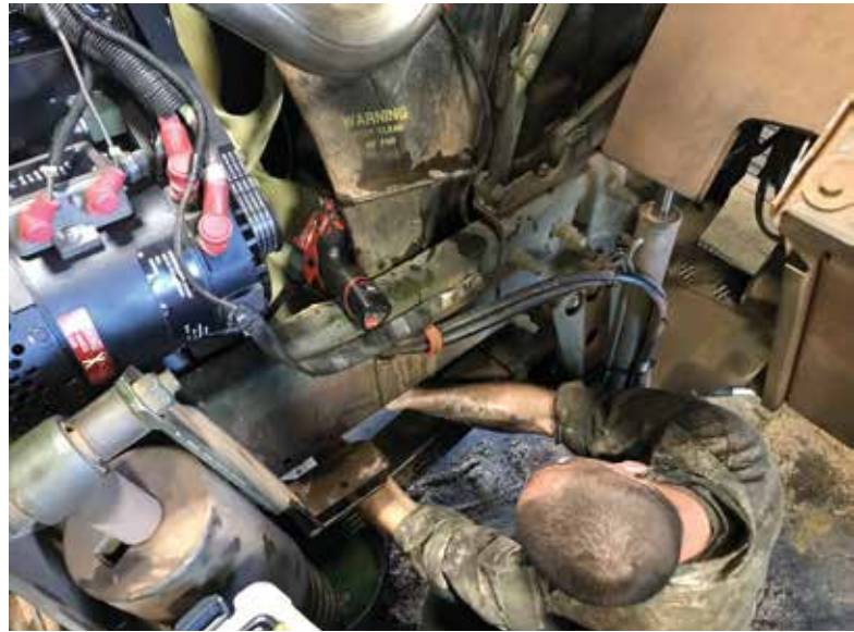
▲ A wheeled vehicle mechanic assigned to the 25th Composite Truck Company, 25th Sustainment Brigade, addresses a radiator hose leak on an FMTV series vehicle, at Schofield Barracks, Hawaii, on 30 May 2018. [US Army]
