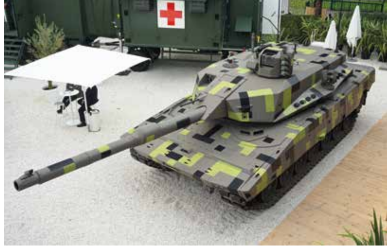
▲ The KF51-U prototype, armed with Rheinmetall's 130 mm gun integrated with their Concept Uncrewed Turret (CUT), was displayed at the Rheinmetall stand at Eurosatory 2024. [RecoMonkey]
