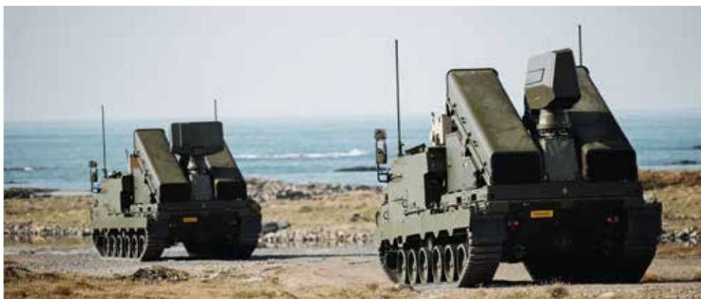
▲ Another trend away from bespoke design is utilising air-to-air missiles shared with air forces for ground-launch use from SAM systems. NOMADS (pictured here) is stated to be able to launch both IRIS-T SLS and AIM-9X. [Kongsberg]
