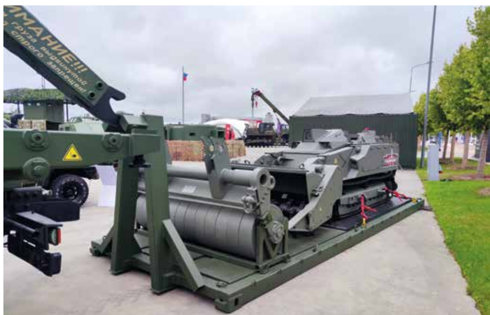
▶ An Uran-6 remotely operated mine-clearing vehicle, used to detect and neutralise explosive threats on the battlefield. [Alexey Tarasov]
